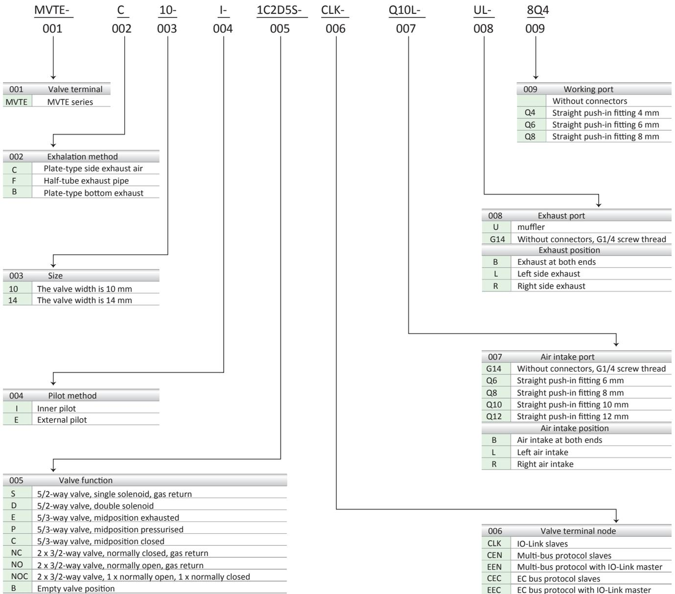
Note: For the 10 mm valve with a wide body, the Q8 type of working interface cannot be selected.
